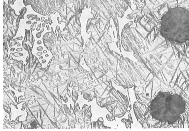
Fig 4 Beneath Barrel SG-P >3%Ni Magnification 200x
