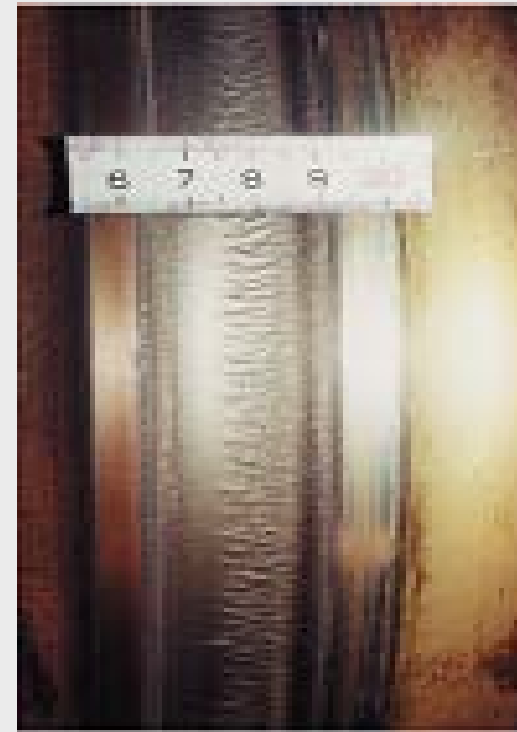
HSS Roll Centrifugal Casting (Rolling amount:1,208ton)
