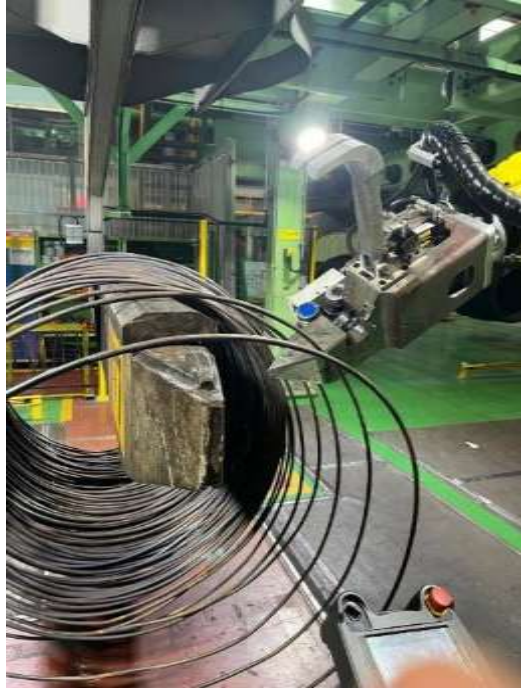
Ring notches and vision identifying where to trim
