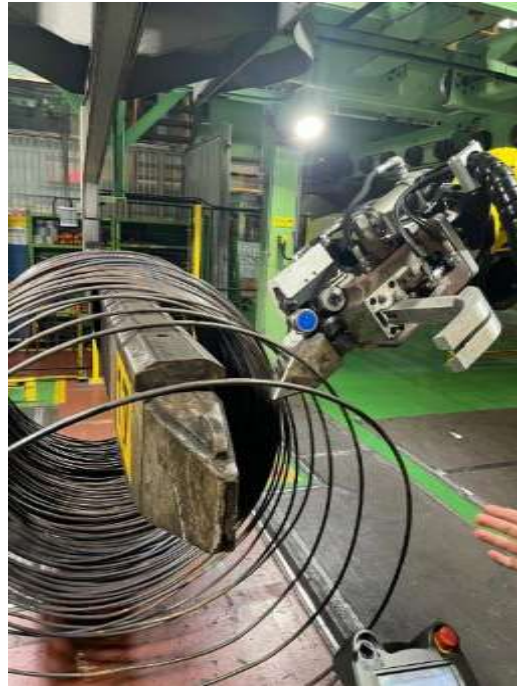
Location to trim is identified and tool inserted
