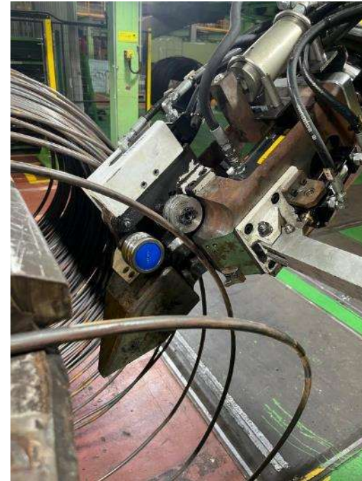
Locating tool between the pinch tools to start the cut
