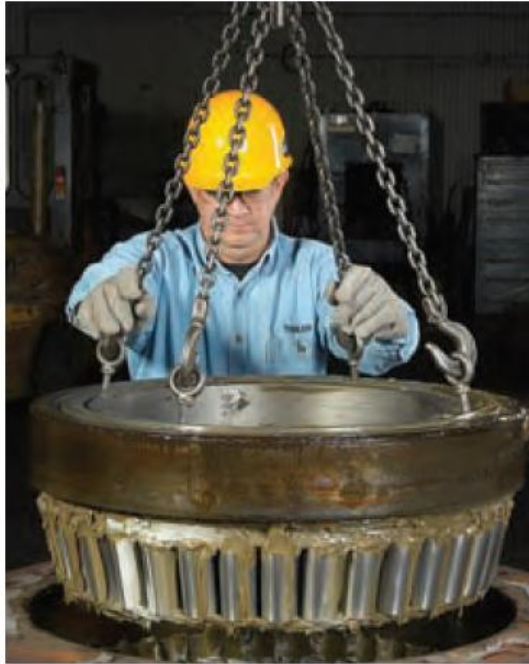
Fig. 8 Remove the top single cup and double cone
