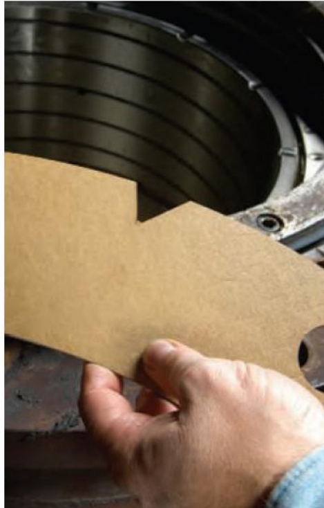
Fig. 39 Notch the gasket
