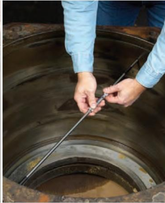
Fig. 24 Check for chock bore size and out-of-roundness
