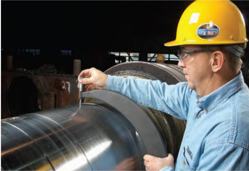
Fig. 41 Before mounting the bearing, check the roll neck for size
