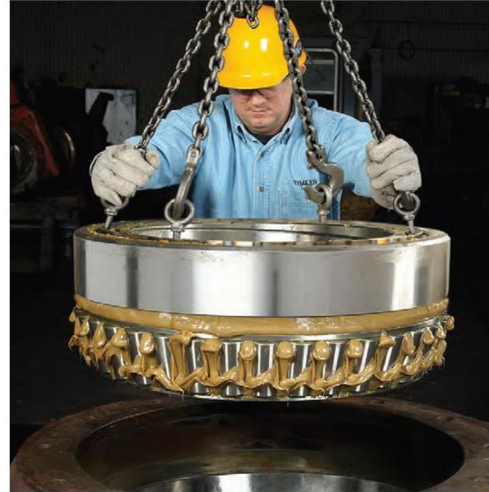
Fig. 38 The top double cone and cup are the last components to be installed into the chock
