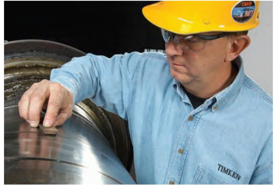
Fig. 42 Remove any nicks or gouges on the roll neck
