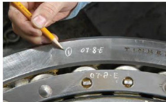
Fig. 31 Each cup quadrant is specified on the bearing
