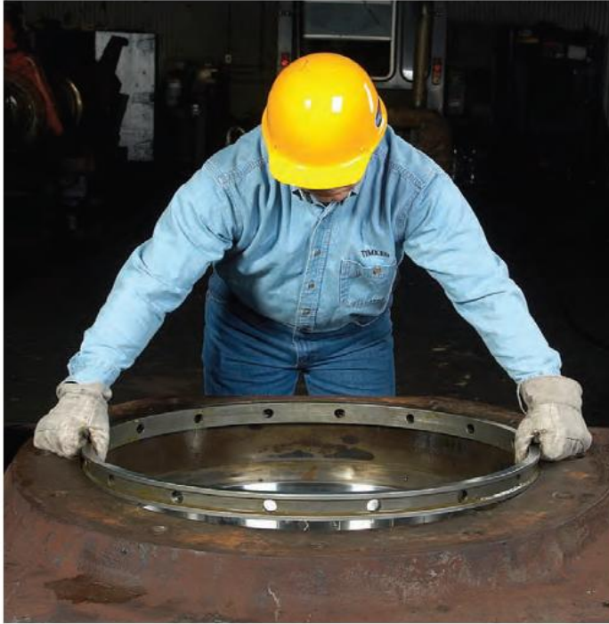
Fig. 37 Place the cone spacer and top cup spacer into position
