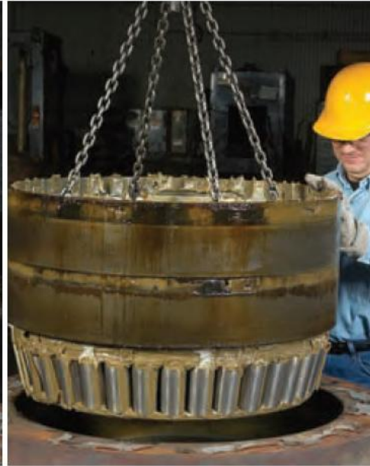
Fig. 9 Remove the double cup, bottom double cone, cone spacer and top cup spacer
