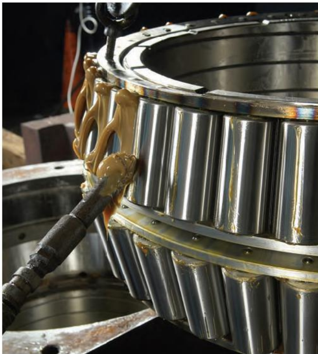
Fig. 35 Lubricate the bearing with grease
