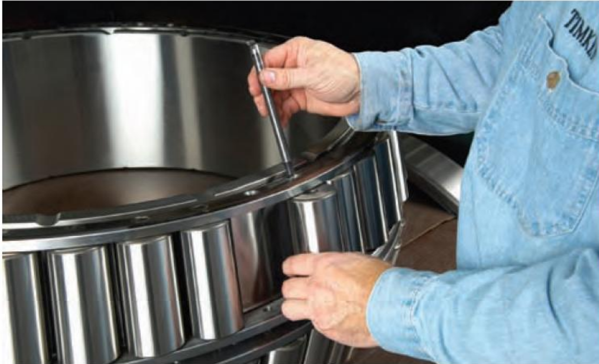
Fig. 12 Remove the roller to inspect the bearing raceway for damage
